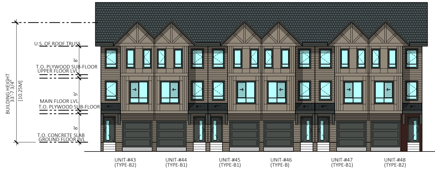
1 ELEVATION AT GARAGE SIDE FACING SCALE 1/16"=1'-0"
