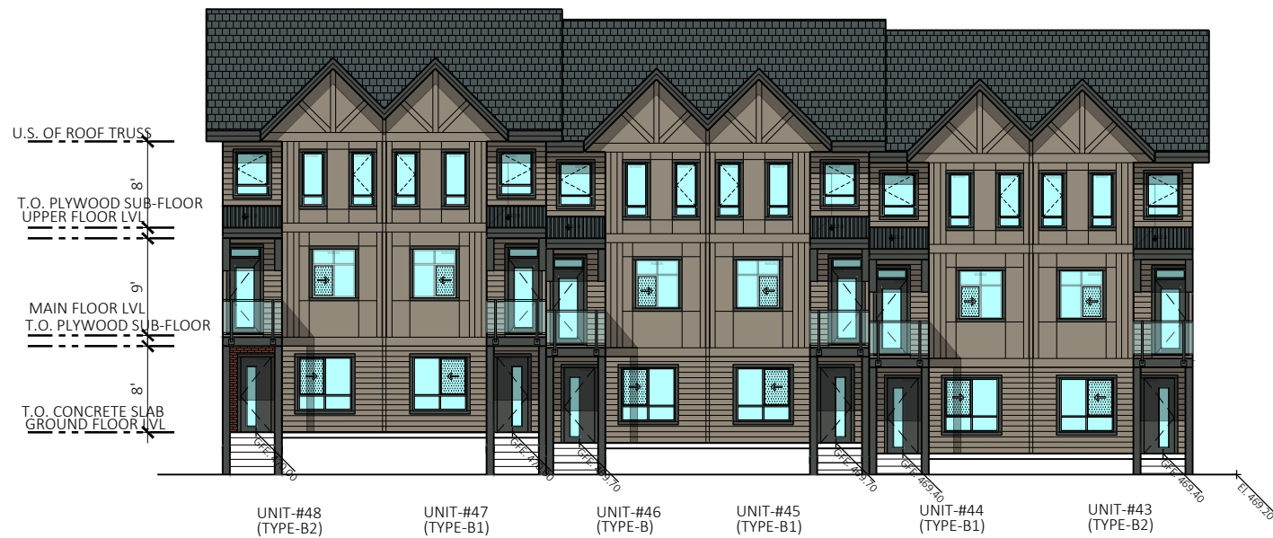
2 ELEVATION AT PRIMARY ENTRY FACING SCALE 1/16"=1'-0"
