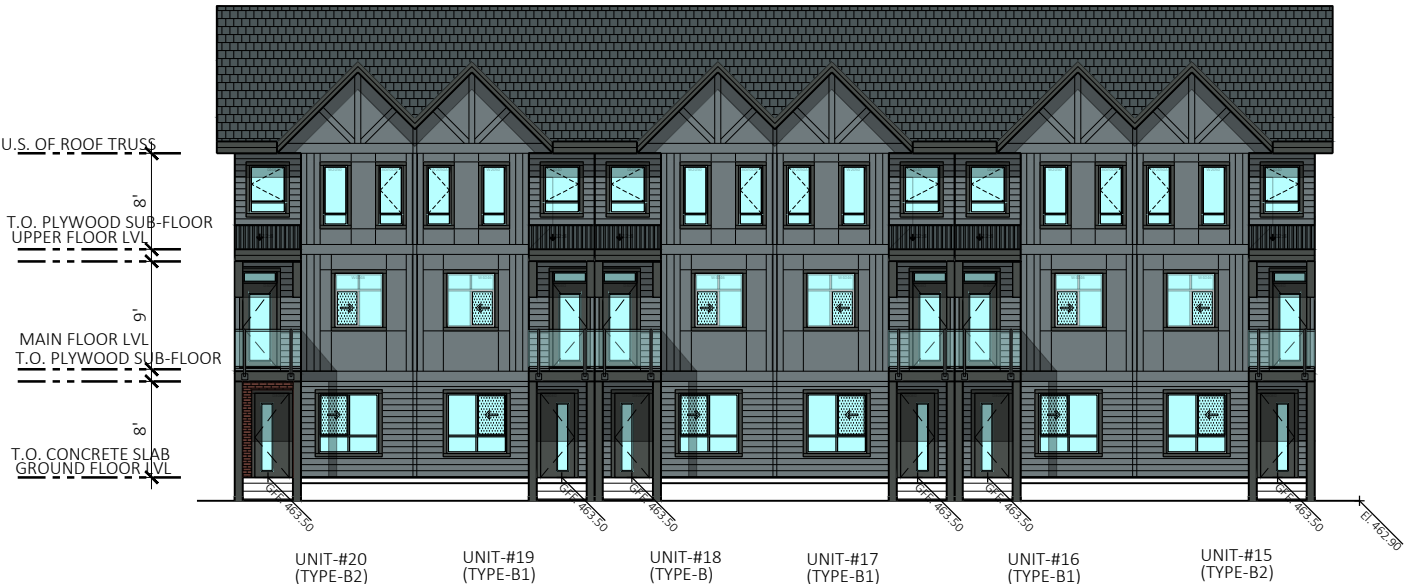
2 ELEVATION AT PRIMARY ENTRY FACING SCALE 1/16"=1'-0"
