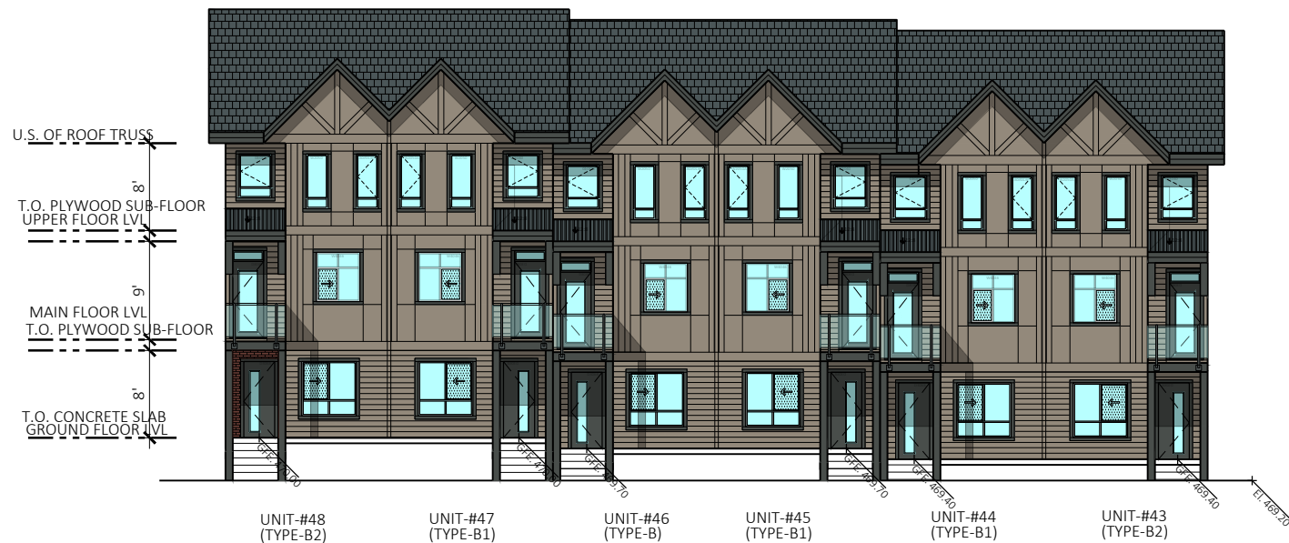
2 ELEVATION AT PRIMARY ENTRY FACING SCALE 1/16"=1'-0"
