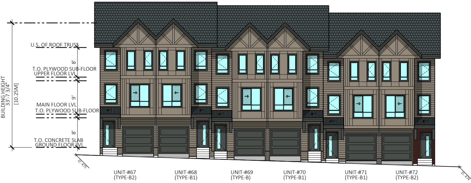
1 ELEVATION AT GARAGE SIDE FACING SCALE 1/16"=1'-0"
