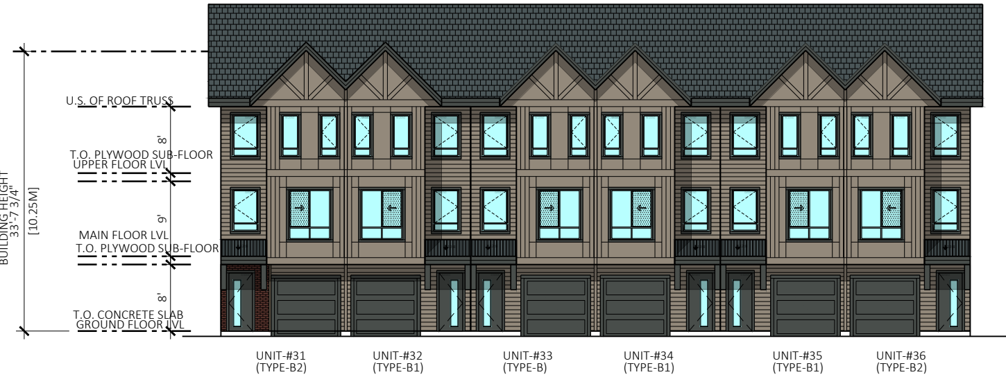
1 ELEVATION AT GARAGE SIDE FACING SCALE 1/16"=1'-0"
