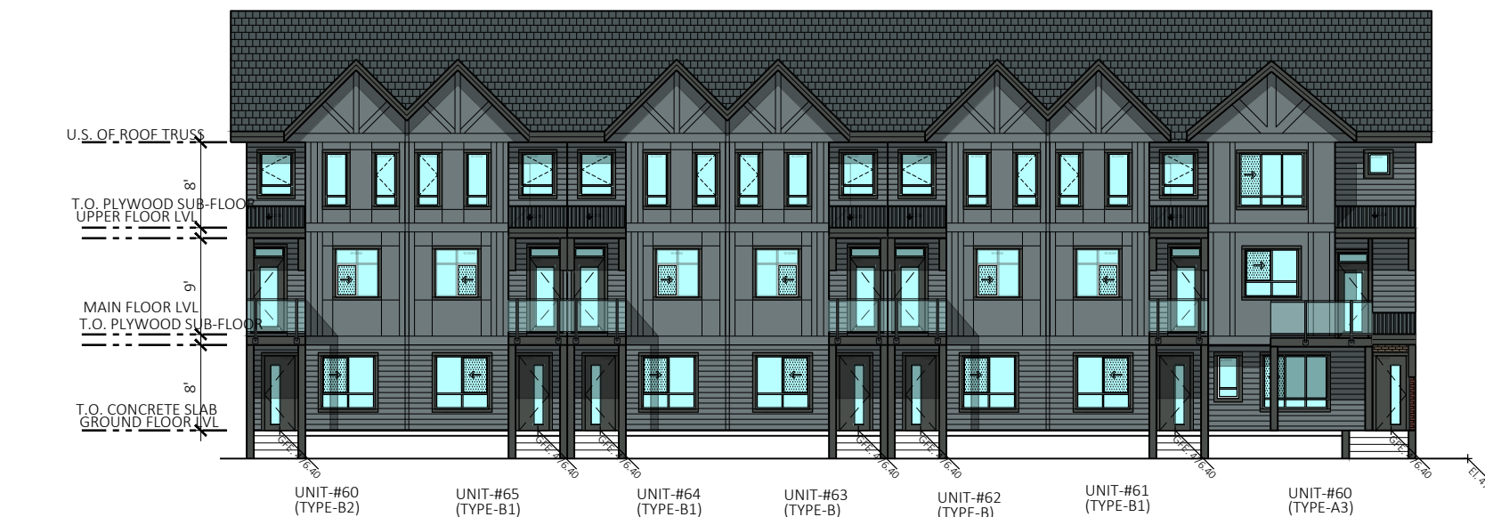
1 ELEVATION AT GARAGE SIDE FACING SCALE 1/16"=1'-0"
