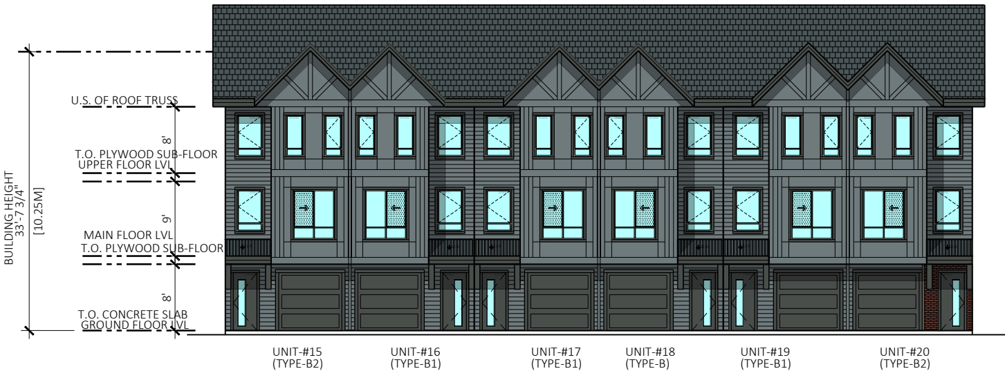
1 ELEVATION AT GARAGE SIDE FACING SCALE 1/16"=1'-0"
