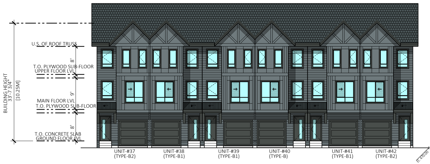
1 ELEVATION AT GARAGE SIDE FACING SCALE 1/16"=1'-0"
