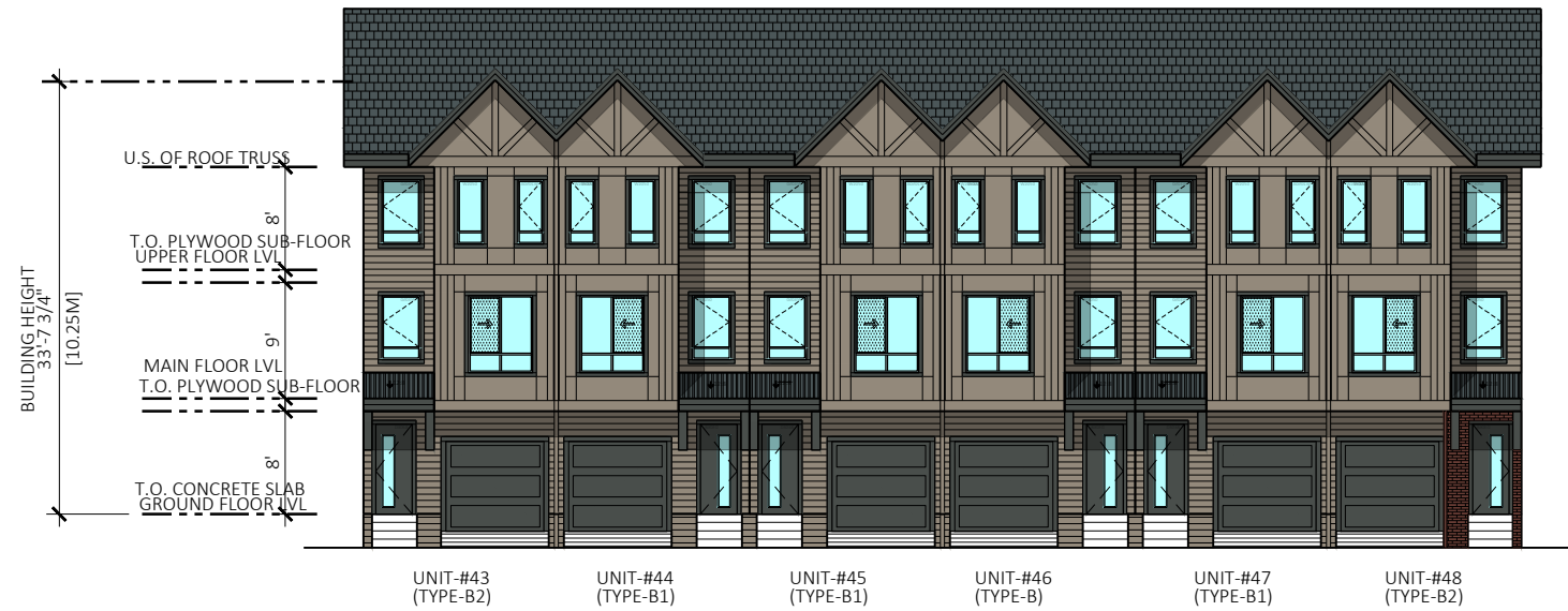
1 ELEVATION AT GARAGE SIDE FACING SCALE 1/16"=1'-0"
