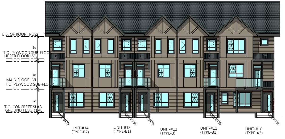
2 ELEVATION AT PRIMARY ENTRY FACING SCALE 1/16"=1'-0"
