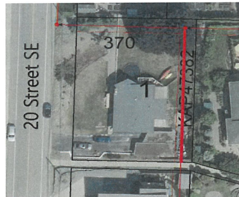
Figure 1- Sanitary Sewer line Requiring Upgrade
