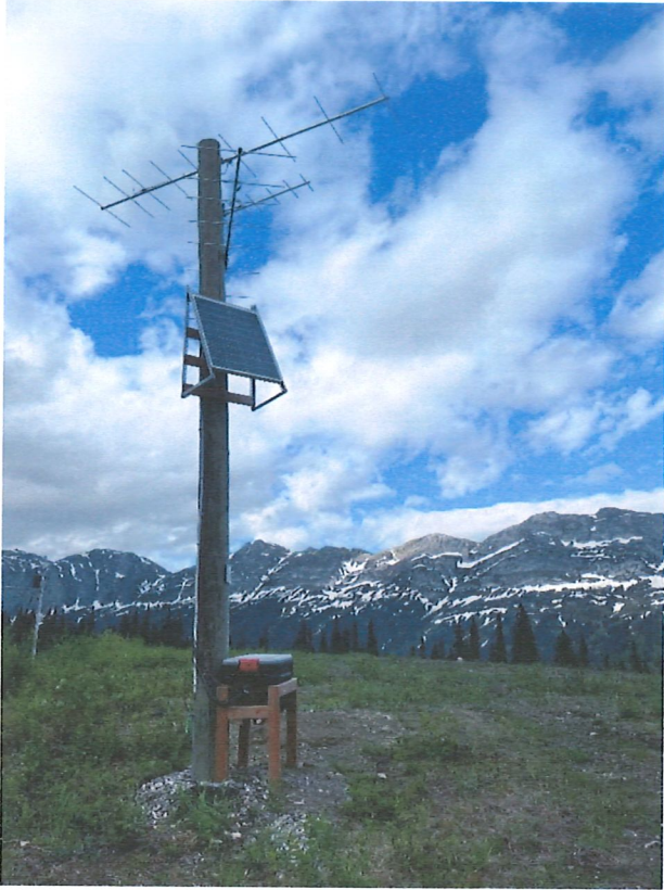
Motus station using a repurposed utility pole in the Pine Pass, BC.
